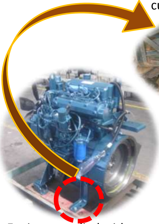
Engines supplied with four transportation feet.
